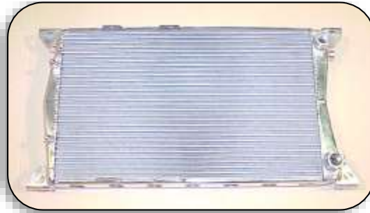
Radiator Lay Flat Type with no cap provision. 1 1/4" Inlet and outlet and has vent port. All aluminum construction. 330mm Wide x 630mm Long PN 40577-00002
