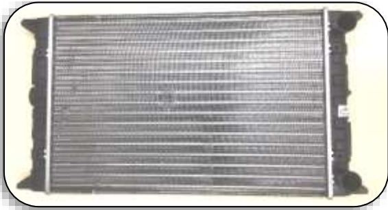
Radiator Lay Flat Type with no cap provision. 1 1/4" Inlet and outlet and has vent port. Plastic Tanks 330mm Wide x 630mm Long PN 40577-00001
